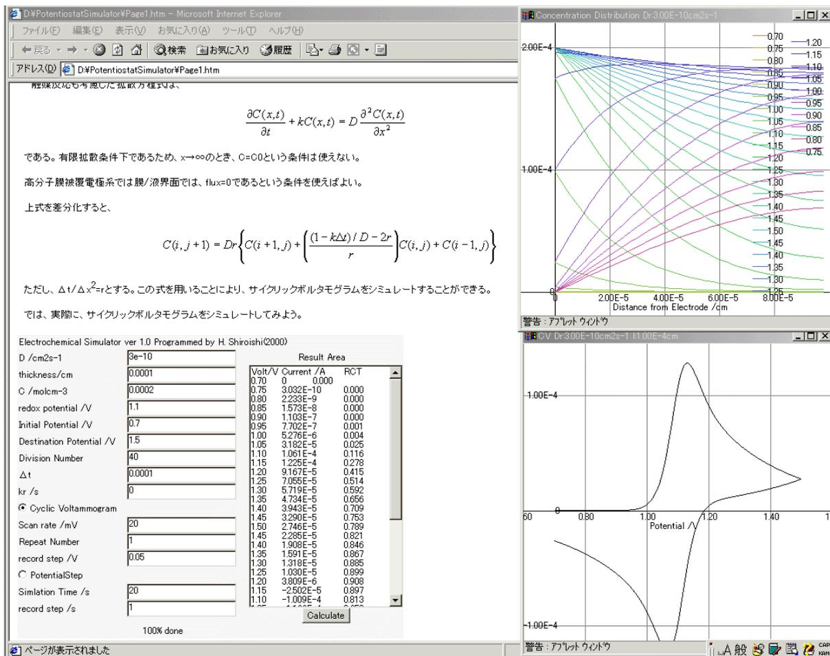
Figure 2. Combination of the ES-1 and electrochemical texts written in HTML. Upper window illustrates the concentration distribution of the oxidized molecule. Lower window shows the cyclic voltammogram of the molecule.
