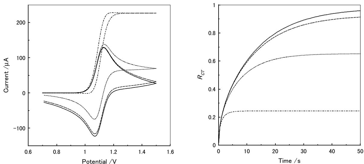
Figure 5. Virtual electrochemical measurements of a material ( $D = 3 \times 10^{-10} \text{cm}^2 \text{s}^{-1}$ ,  $E^\circ = 1.1 \text{V}$  vs. a standard electrode) at various  $k$  values using ES-1. —,  $k = 0 \text{s}^{-1}$ ; - - -,  $5 \times 10^{-3} \text{s}^{-1}$ ;  $\cdots$ ,  $5 \times 10^{-2} \text{s}^{-1}$ ; - · - ·,  $5 \times 10^{-1} \text{s}^{-1}$ . (a) Cyclic voltammogram from 0.7 V to 1.5 V at 20mV/s. (b) Time dependence of  $R_{CT}$  at an applied potential from 0.7V to 1.5V.
