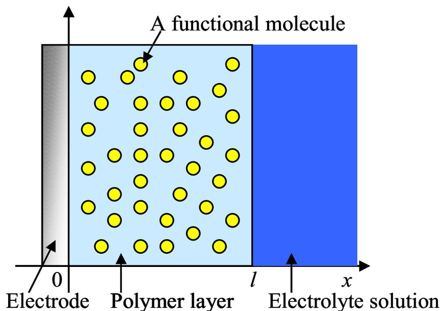
Figure 1. Scheme of a polymer-coated electrode with dispersed functional molecules
