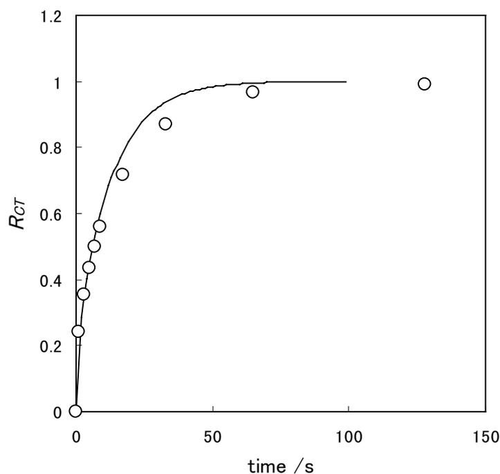
Figure 3. Time dependence of  $R_{CT}$  estimated by absorption spectral change at potential step measurement from 0.6V (versus Ag|AgCl) to 1.4V using ITO/Nafion[Ru(bpy)<sub>3</sub><sup>2+</sup>] electrode in 0.1 mol dm<sup>-3</sup> KNO<sub>3</sub> (pH 1). The solid line was calculated with ES-1. ( $D = 3.2 \times 10^{-10}$  cm<sup>2</sup>s<sup>-1</sup>,  $l = 1 \times 10^{-4}$  cm,  $C_T = 4.2 \times 10^{-4}$  mol cm<sup>-3</sup>)
