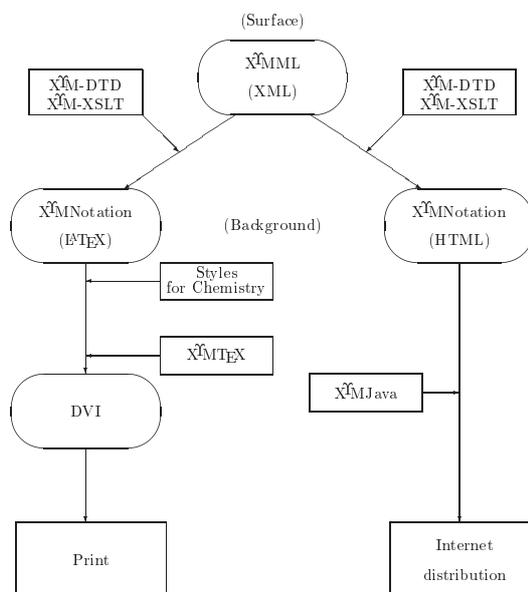
Figure 1. X<sub>Y</sub>M<sub>T</sub>E<sub>X</sub> as part of a communication system of chemical documents. The acronym “DVI” means a “device-independent” file produced by a T<sub>E</sub>X/L<sub>A</sub>T<sub>E</sub>X processing.
