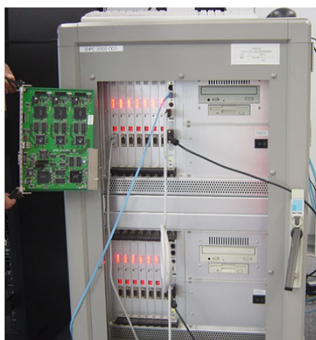
Figure 1. EHPC SH4 processor board (left) and platform system (2-unit in picture).
