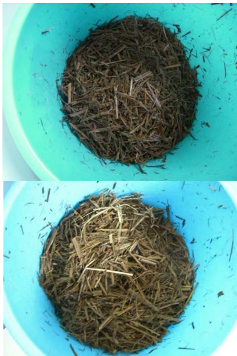
Figure 4: Residues from rice straw (a: saccharification treatment, b: alcohol fermentation treatment)
