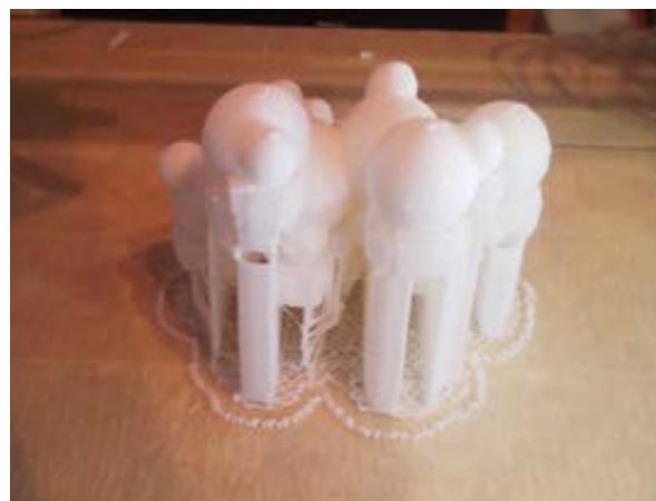
Fig.13 3D molecular model of glucose that has just been printed
