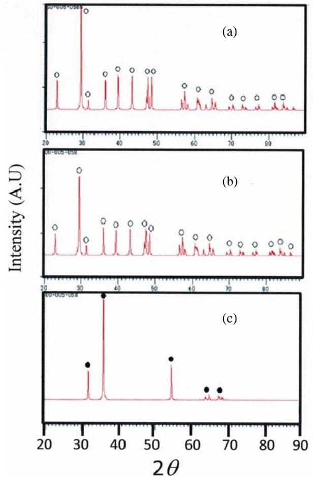
Fig. 3. XRD patterns for PSU-shell fired at (a) 600, (b) 800, and (c) 1000 °C. ○CaCO<sub>3</sub>, ●CaO.
