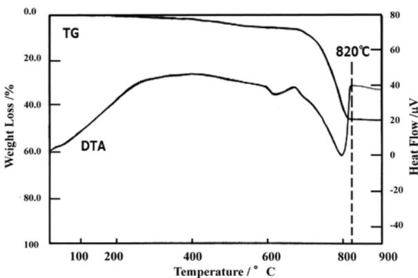
Fig. 2. TG and DTA profiles for PSU powder.
